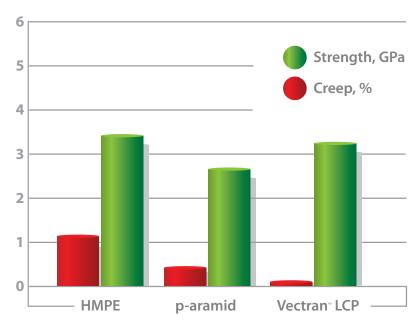
Source: Internal testing or published data. Creep conditions 25°C, 30% load, 100 hrs.
